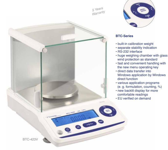
Internal Calibration 2 seconds measuring time
