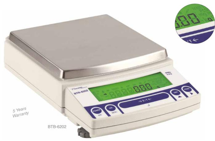
External Calibration 3 seconds measuring time
